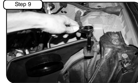
With 10mm socket or wrench, tighten down housing using provided M6 screw.
