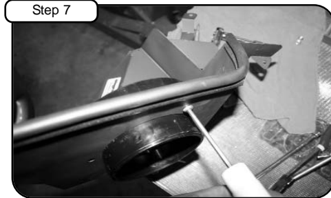
Place trim seal on top of new housing. With 5 1/2" adapter, place inside of new housing with 3 button head screws provided, tighten with 5/32" allen key.
