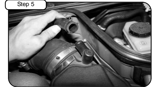
Disconnect the factory crank case line from OEM intake tube. Disconnect MAF sensor wire harness from intake.
